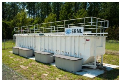
Figure 1: Radionuclide Field Lysimeter Experiment (RadFLEx) at the USDOE Savannah River Site.
